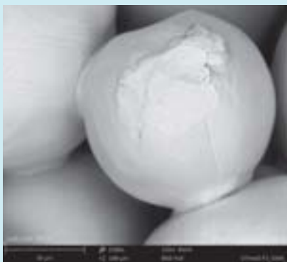
Abb.2 Gesintertes OT-F 3 Implantat, OT medical (2500x)
